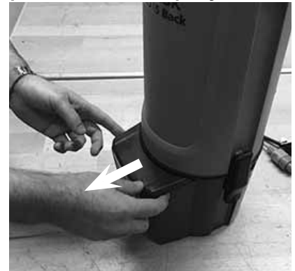
HEPA exhaust filter to be replaced once/twice per year
