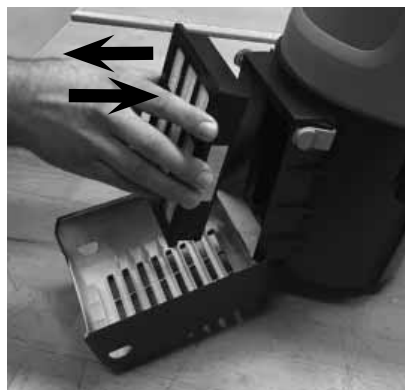
Pre filter to be replaced by use of every 5-10 dust bags
